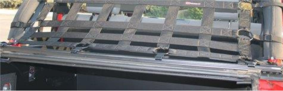
Next, working your way up the back of the cage, attach the hooks in the existing cut outs on the rail of your jeep. Do not tighten buckle just yet.
