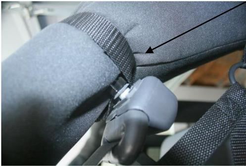
Then continue all the way to the front, attaching all the straps on the roll bar, but do not tighten.
