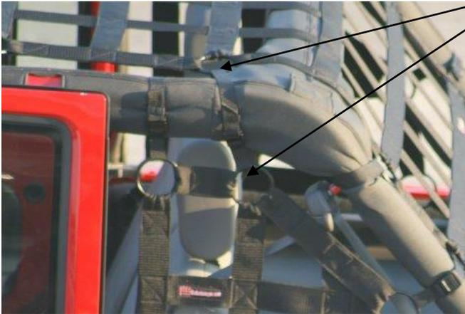
The front corner straps slip underneath the plastic cover in the corner and tie around the metal roll bar.
