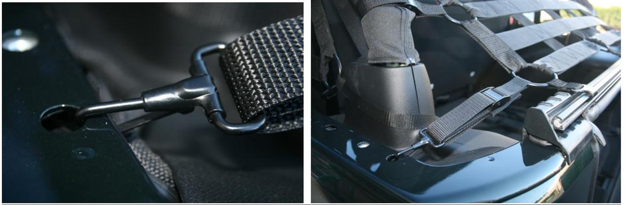
Attach the next strap around the roll bar just above the plastic seatbelt retainer box. Now adjust and tighten this strap on both sides. Then adjust and tighten the strap just below with the hook, both sides.
